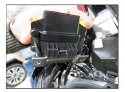
7) Using 2 of the supplied combination tie strap/clip retainers, route and secure as shown in figure TBD.
