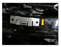
6) After you have installed the bracket, attach the relay box to the bracket mount
