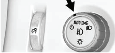
Exterior Lamp Controls here
