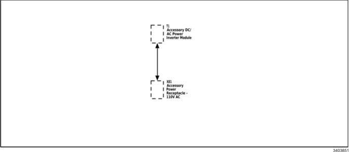
The alternating current (AC) accessory power outlet system consists of the accessory DC/AC power inverter module and the accessory power receptacle -110 V AC. The accessory DC/AC power inverter module converts 12 V direct current (DC) battery power to 110 V at 60 Hertz (Hz) AC power to operate AC powered devices. The accessory DC/AC power inverter module provides up to 150 watts of power. The accessory power receptacle -110 V AC provides the usual connection for AC powered devices.
