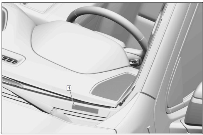
The vehicle identification number (VIN) plate (1) is the legal identifier of the vehicle. The VIN plate is located on the upper left corner of the instrument panel. The VIN number can be seen through the windshield from the outside of the vehicle:
