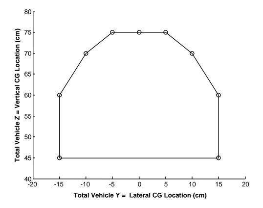
For upfitter use and applicable to CMVSS 126 and FMVSS 126, the longitudinal and vertical vehicle center of gravity location can be approximated by following the formula below and by referencing data elements within CMVSS 105 and FMVSS 105 – HYDRAULIC AND ELECTRIC BRAKE SYSTEMS or CMVSS 135 and FMVSS 135 LIGHT VEHICLE BRAKE SYSTEMS, ... ALLOWABLE CENTER OF GRAVITY CHARTS.
