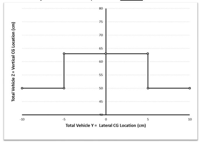
For upfitter use and applicable to CMVSS 126 and FMVSS 126, the longitudinal and vertical vehicle center of gravity location can be approximated by following the formula below and by referencing data elements within CMVSS 105 and FMVSS 105 – HYDRAULIC AND ELECTRIC BRAKE SYSTEMS or CMVSS 135 and FMVSS 135 LIGHT VEHICLE BRAKE SYSTEMS, ... ALLOWABLE CENTER OF GRAVITY CHARTS.
