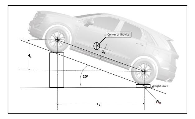
3. The <u>vertical</u> center of gravity location  $Z_0$  is determined by:
