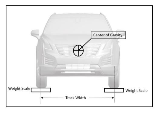
For all types of incomplete vehicles contained in this document with an average front track of 1587 mm (62.47 in), the <u>lateral</u> center of gravity location is determined by:
