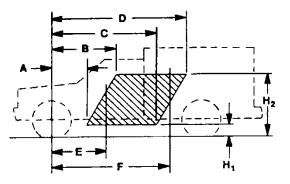
C/G of vehicle in CMVSS or FMVSS unladen condition [Curb + 181.4 kg. (400 lb.)] must be inside shaded area – that is, the C/G must be within the trapezoid formed by the coordinates A, B, C, D, H1, & H2, plus the C/G must be to the rear of vertical line E and forward of vertical line F.
