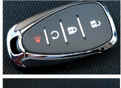
The Keyless Access system allows for the vehicle entry when the remote is within 3 ft (1 m)
