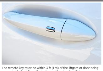
opened or locked. Press the button on the door handle to open.
