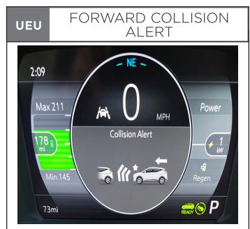
The Forward Collision Alert (FCA) system may help to avoid or reduce the harm caused by front-end crashes. with detected vehicle being followed. When approaching a vehicle ahead too quickly, FCA provides a red flashing alert on the windshield and rapidly beeps. FCA also lights an amber visual alert if following another vehicle much too closely. FCA detects vehicles within a distance of approximately 60m (197 ft) and operates at speeds above 8 km/h (5 mph).
