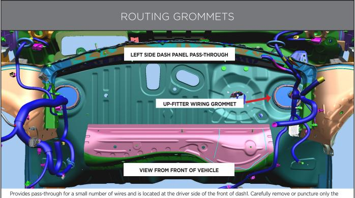
portion required for the passage of upfitter wires and silicone seal around the wires after installation. Note that a vehicle harness is passing through the grommets and care must be taken to avoid damaging these harnesses especially in the instrument panel interior.
