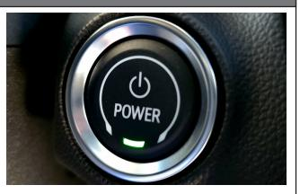
If key fob not detected, from low fob battery, or radio interference, hold key to start button to start
