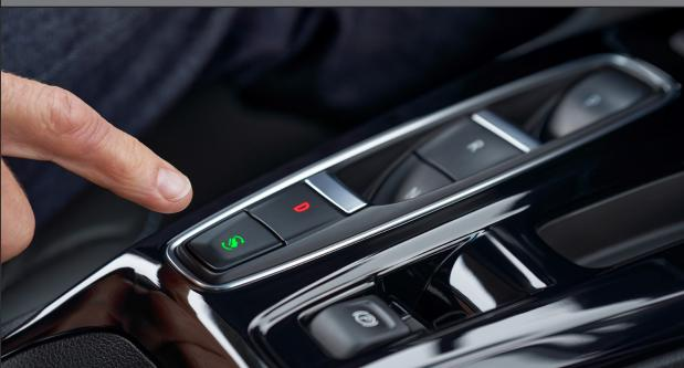
This vehicle is equipped with an electronic transmission. The shift switches are designed to prevent inadvertent shifting out of Park (P) unless the ignition is on and the brake pedal is applied. Push/Pull-to-shift transmission technology is intuitive to use, with pull switches for Drive (D) and Reverse (R) and push switches for Park (P), and Neutral (N). Note: While in Accessory power mode with the brake pedal pressed the vehicle can be shifted only into Neutral (N) from Park (P).
