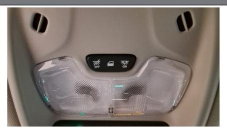
There are dome lamps in the overhead console and the headliner. To change the dome lamp settings, activate the following: - Press OFF to tum off the dome lamps when a door is open.
