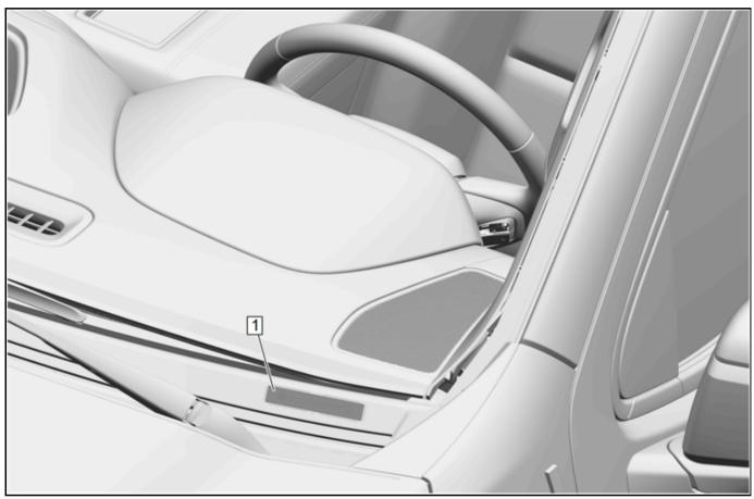
The VIN plate is the legal identifier of the vehicle. The VIN plate is located on the upper left corner of the instrument panel (I/P) and can be seen through the windshield from the outside of the vehicle:
