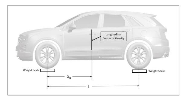
3. The **longitudinal** center of gravity location, X<sub>0</sub>, is determined by:
