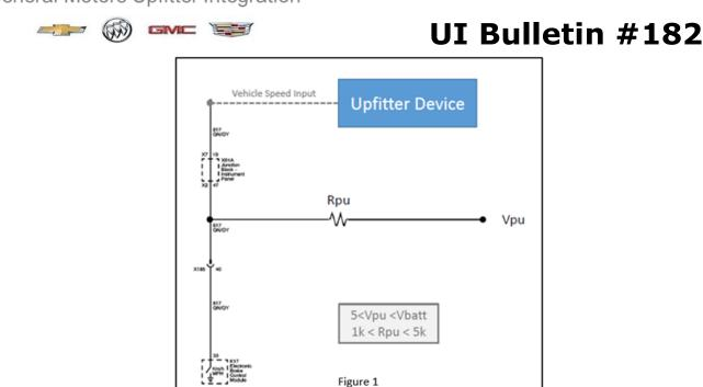
If the VSS as provided and the use of V+ mechanization shown in Figure 1 is not a viable option to obtain a V+ pulse required by the added equipment then the vehicle may be rewired as outline in the steps below to obtain the VSS from the TCM as was provided in previous model years.
