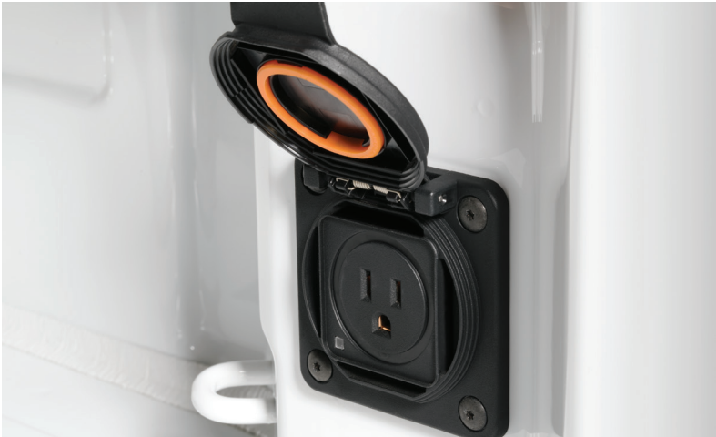
Standard 120-volt power outlet in bed
