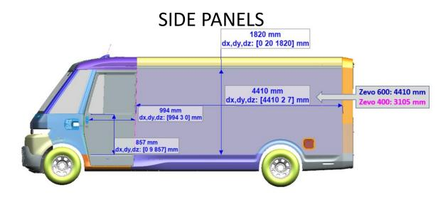
The only difference between ZEVO 400 and ZEVO 600 is the length of the cargo side panel & roof panel. Please see pic. The rest of the dimensions (front, side, & rear) are the same as ZEVO
