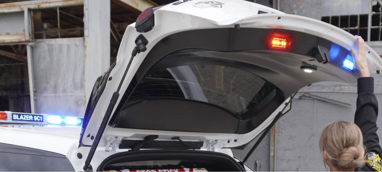
T53 REAR LIFTGATE WARNING LIGHTS
