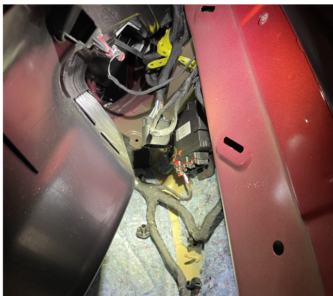
Module and user harness located right rear interior quarter panel.
