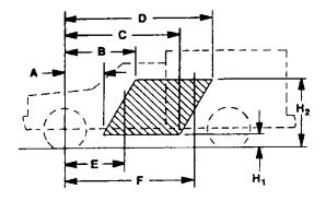
C/G of vehicle in CMVSS or FMVSS unladen condition [Curb + 181.4 kg. (400 lb.) or Curb + 226.8 kg. (500 lb.) as defined by CMVSS 105 and FMVSS 105] must be inside shaded area – that is, the C/G must be within the trapezoid formed by the coordinates A, B, C, D, H1, & H2, plus the C/G must be to the rear of vertical line E and forward of vertical line F.
