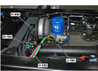
Connectors are located between the frame rails, on the crossmember next to the fuel tank.
