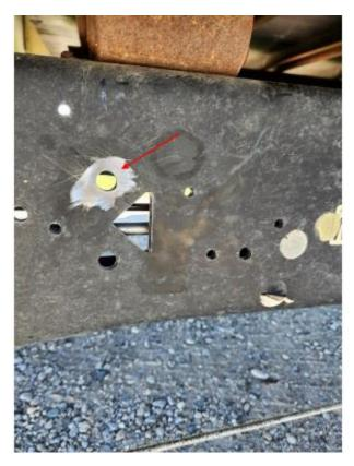
Attach end of ground cable to the vehicles frame and secure cable.
